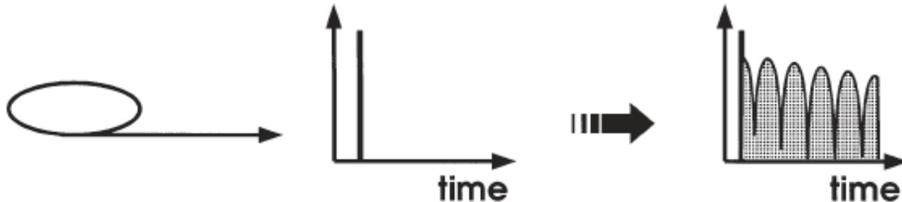
Figure 1. Reciprocal properties of radioactive sources (top) and synchrotron radiation (bottom) lead to reciprocal experimental techniques. The center panels illustrate the source characteristics averaged over a time period needed for data collection.
