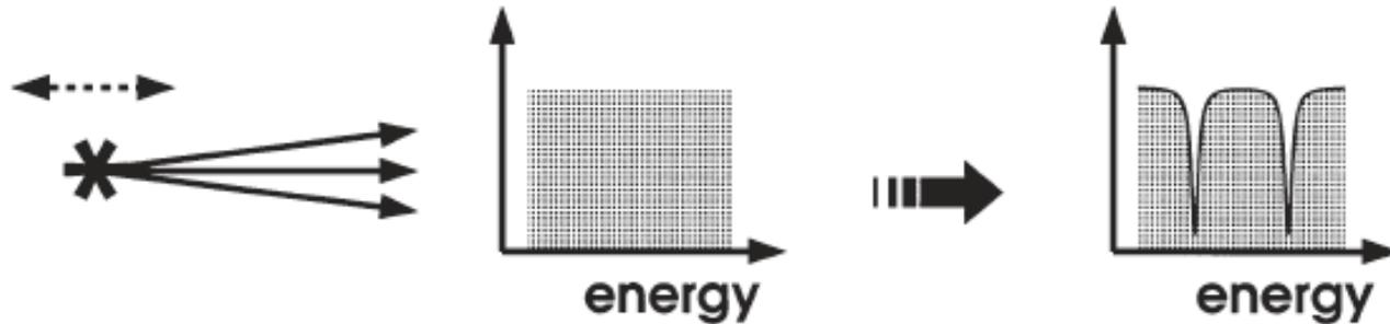
Time-resolved spectroscopy (Synchrotron)
